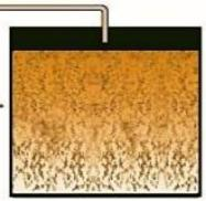
3. Settling: heavier bio mass sinks to the bottom & mud stabilization
