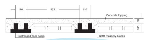
a) Prestressed beam - Grade 40/14 concrete.
