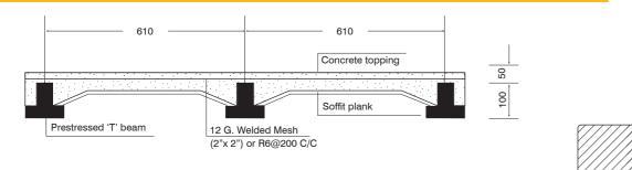
a) Prestressed beam - Grade 40/14 concrete.
