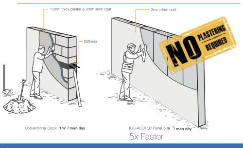
\*BUILDABILITY is the extent to which the design and the adoption of construction techniques & processes affects the productivity level of building works
