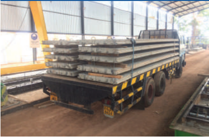
Prestressed Floor Slab
